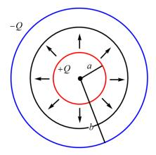
integrate both sides of equation (1) over the volume of a concentric sphere with radius r, where a < r < b. The black arrows indicate the electric field vectors.
