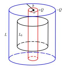
integrate both sides of equation (1) over the volume  $V_0$  of a coaxial cylinder with radius r, where a < r < b, and length  $L_0$ . The electric field vectors point radially outward because otherwise charges would accelerate in the cylinders.
